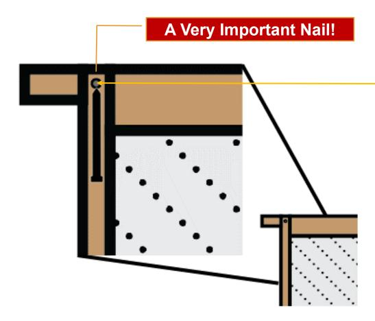
It can be placed through the end bar, just under the ear of the top bar so the nail locks into the top bar (*right*)
